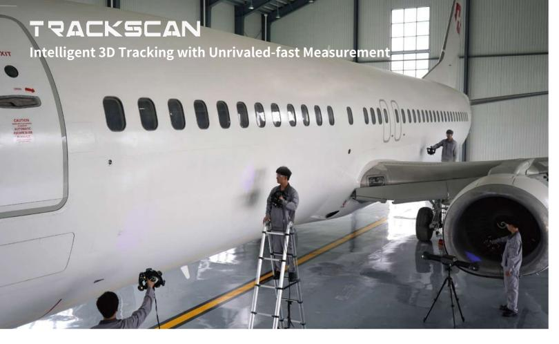
TrackScan-P42 adopts intelligent optical tracking measurement technology and high-quality optical equipment, carrying out ultra-high precision dynamic 3D measurement without markers.
