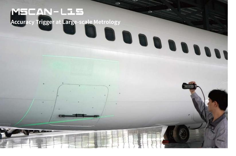
MSCAN-L15 photogrammetry system is tailored to deliver high-precision geometric measurements of large-scale workpieces. With a large shooting area and wide depth of field, it performs volumetric accuracy of 0.015 mm/m for large-scale projects.
