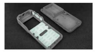
Maciej Burzyński from Sybet prototyped with Sinterit Lisa a portable handheld receiver for KGHM, the world leader in copper and silver production. Printing the whole set of radiotelephone parts with PA12 and Flexa Grey costs less than 600 USD and takes about four days.
